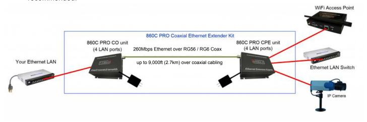
The Overview Diagram: This diagram shows the contents of the product box inside the rectangle. Devices outside the rectangle above are your equipment that can be attached.
