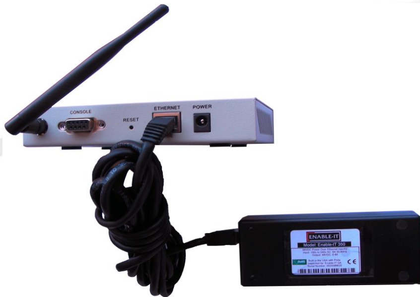
Figure 1 Enable-IT 350 to a 8424 WiFi PoE Access Point
