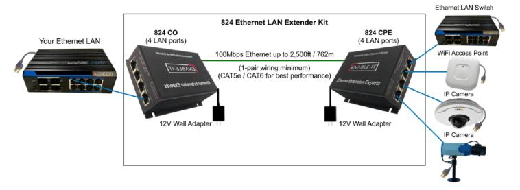
The Overview Diagram: This diagram shows the contents of the product box inside the rectangle. Devices outside the rectangle above are your equipment that can be attached.
