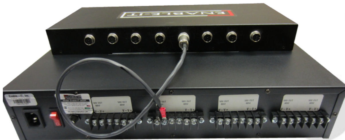
8955M Port 5 Secure Locking PoE input connected to 3600R
