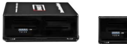
Default DIP settings 865 CPE – All down set in the ON position 865 CO – DIP position 1 up (OFF) DIPs 2-4 down (ON)
