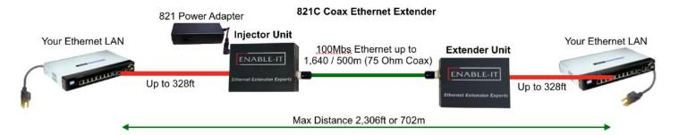
We highly recommend that you perform a quick out of the box test to ensure the working order of your Enable-IT 821C Coax Ethernet Extender units prior to installing. This will also serve to familiarize you with how easy the process should be. Follow the steps below to perform the Out Of the Box Test.
