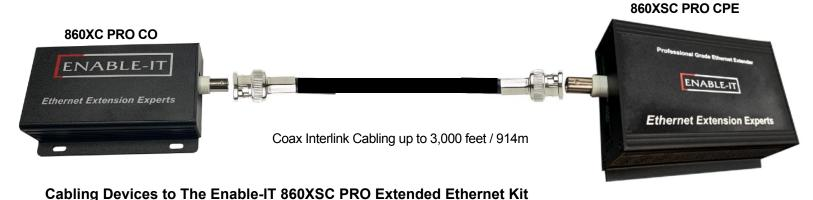
Attach your remote LAN device to the 860XSC PRO CPE unit LAN ports with Ethernet patch cord provided. Attach your local LAN to the 860XSC PRO CO LAN ports with Ethernet patch cord provided. Attach the power adapters to both 860XSC PRO units.
