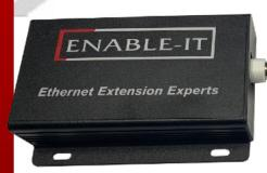
The 860XSC PRO Coax quad LAN port enables the simple installation of a high speed Ethernet backbone at distances up to 3,000ft / 915m using 75 Ohm RG-6 coax with BNC connectors.
