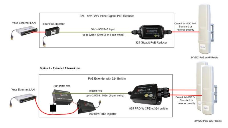
Keep in mind that Ethernet data has a limit of 328ft or 100m. You can easily solve this issue by using the Enable-IT 324W PoE Reducer with an Enable-IT 865 PoE Ethernet Extender kit. Using the 865 kit will drive your PoE and data up to 3,500ft / 1.06km.
