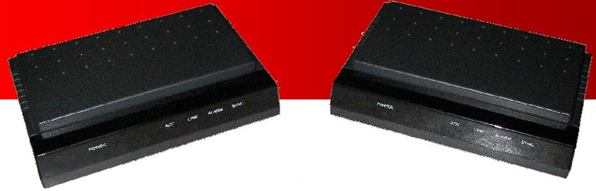
The Enable-IT 890 Series LRE is a unique Ethernet LAN product that leverages digital technology to drive industry standard 10baseT and 100baseT signals to over fifteen times specified Ethernet distances. This cost-effective solution eliminates many of the limitations and high costs for extending LAN cabling today.
