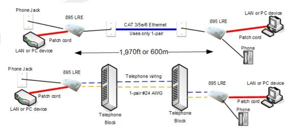
Choose a location to mount each of the Enable-IT 895's where the maximum distance does not exceed 1,970ft or 600m total between devices to be connected.
