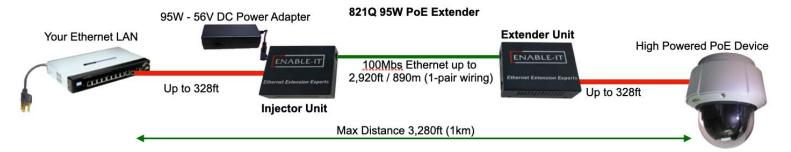
We highly recommend that you perform a quick out of the box test to ensure the working order of your Enable-IT 821Q 95W PoE Extender units prior to installing. This will also serve to familiarize you with how easy the process should be. Follow the steps below to perform the Out Of the Box Test.
