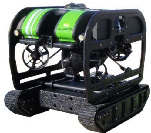
Figure 1. A MiniROV with Crawler Attachment (tracked option). Photo courtesy of SeaBotix, Inc.
