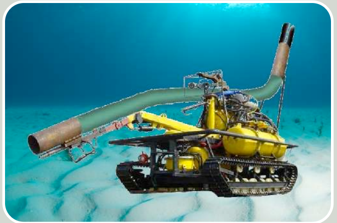
Robotic Seafloor Crawler HiDef PoE IP Camera powered from within the robot umbilical and Ethernet driven from the surface vessel.
